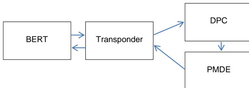
Figure 5.3: PMD test using StrataLight system as a transponder
