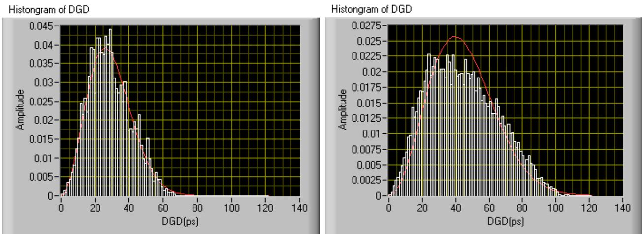
Figure 5.2: (left) DGD Histogram for PMD=10ps (right) DGD Histogram for PMD=16ps
