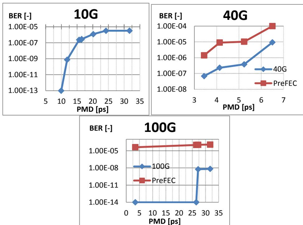
Figure 5.4: BER of telco modulations in presence of PMD: 10G (top left), 40G (top right) and 100G (bottom)
